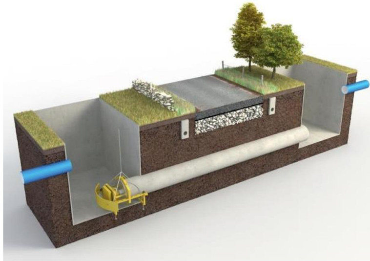
Insert 2-9 – Illustrative example of a Microtunnel Crossing
